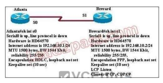
Given the partial configurations, identify the fault on the Brevard router that is causing the lack of connectivity
