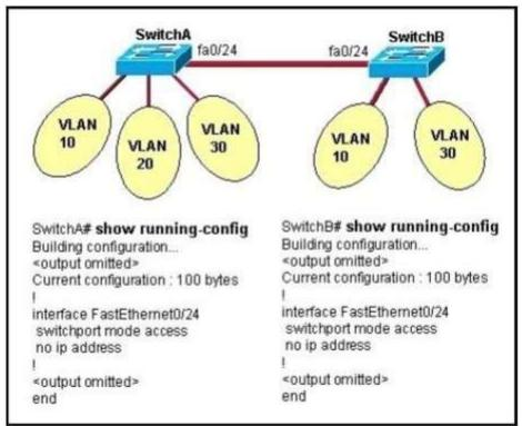
All switch ports are assigned to the correct VLANs, but none of the hosts connected to SwitchA can communicate with hosts in the same VLAN connected to SwitchB. Based on the output shown, what is the most likely problem?
