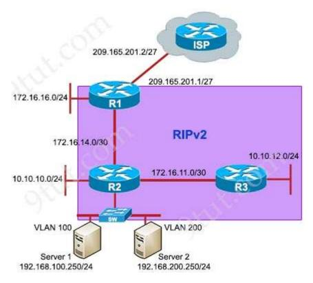
Examine R2 configuration, the traffic that is destined to R3 LAN network sourced from Router R2 is forwarded to R1 instead R3. What could be an issue?
