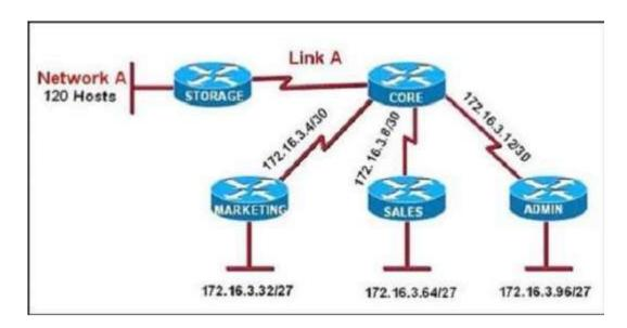
All of the routers in the network are configured with the ip subnet-zero command. Which network addresses should
