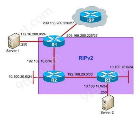
Why applications that are installed on PC's in R2 LAN network 10.100.20.0/24 are unable to communicate with Server1?
