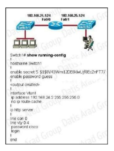
The network administrator cannot connect to Switch 1 over a Telnet session, although the hosts attached to Switch1
